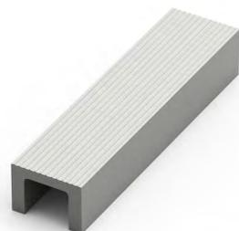
If the front-to-back dimension of the mat well is greater than the final width of your matting, you may need a U section to secure the different sections together. Supplied in sections of 10' (3m) length, with fixing screws and plugs. Comes in anodized aluminum, powder coated dark gray and black. Size: 9/16" x 3/4" (14mm x 19mm)
