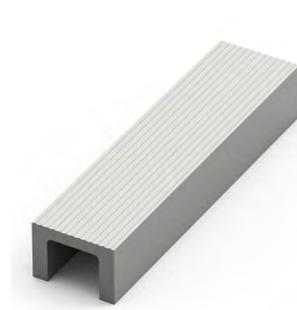
If the front-to-back dimension of the mat well is greater than the final width of your matting, you may need a U section to secure the different sections together. Supplied in sections of 10' (3m) length, with fixing screws and plugs. Comes in anodized aluminum, powder coated dark gray and black. Size: 3/8" x 11/16" (10mm x 18mm)
