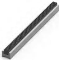
If the front-to-back dimension of the mat well is greater than the final width of your matting, you may need a H section to secure the different sections together. Supplied in sections of 12' (3.6m) length, with fixing screws and plugs. Comes in black, with mat insert colour specified. Size: 9/16" x 1/2" (14mm x 13mm).
