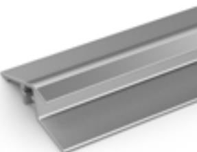
Supplied in sections of 6'6" (2m) length with fixing screws and plugs. Comes in anodized aluminum and powder coated yellow. Size: 9/16" x 1 13/16" x 6'6" (14mm x 45mm x 2m)
