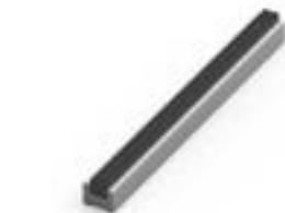
If the front-to-back dimension of the mat well is greater than the final width of your matting, you may need a H section to secure the different sections together. Supplied in sections of 10' (3m) length, with fixing screws and plugs. Comes in black, with mat insert colour specified. Size: 9/16" x 15/32" (14mm x 12mm)
