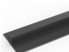
Two-part snap track that can be welded together to join rolls end-to-end or side-to-side to cover large areas. Supplied with cold welding paste. Comes in dark gray. Size: 9/16" x 8'2" (14mm x 2.5m)
